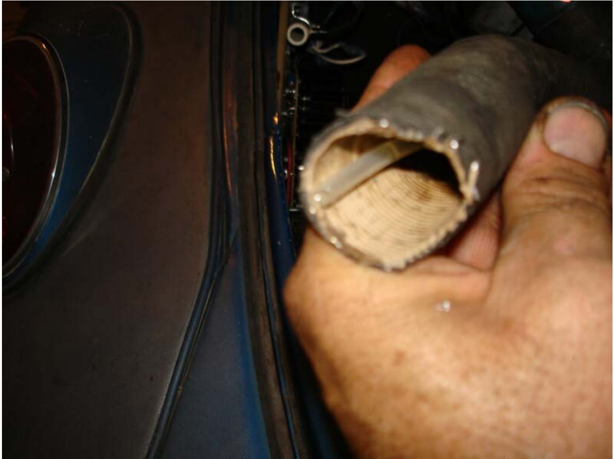
shows the hot exhaust pipe that the water drips onto
