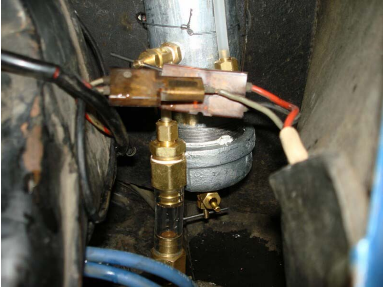
Shows water line entering hot carburetor air inlet tube
