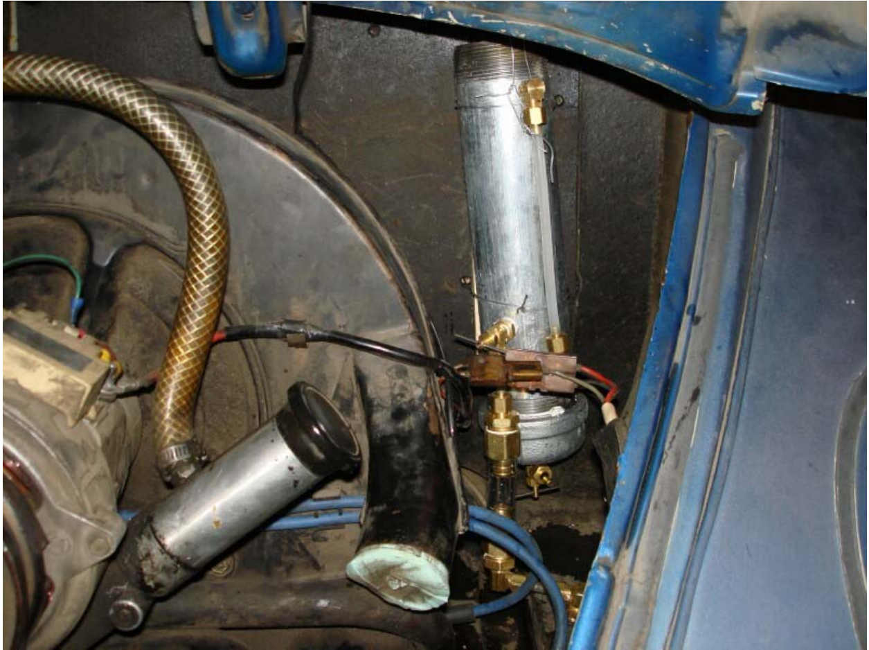
Shows sight glass (vinyl really) & needle valve above
